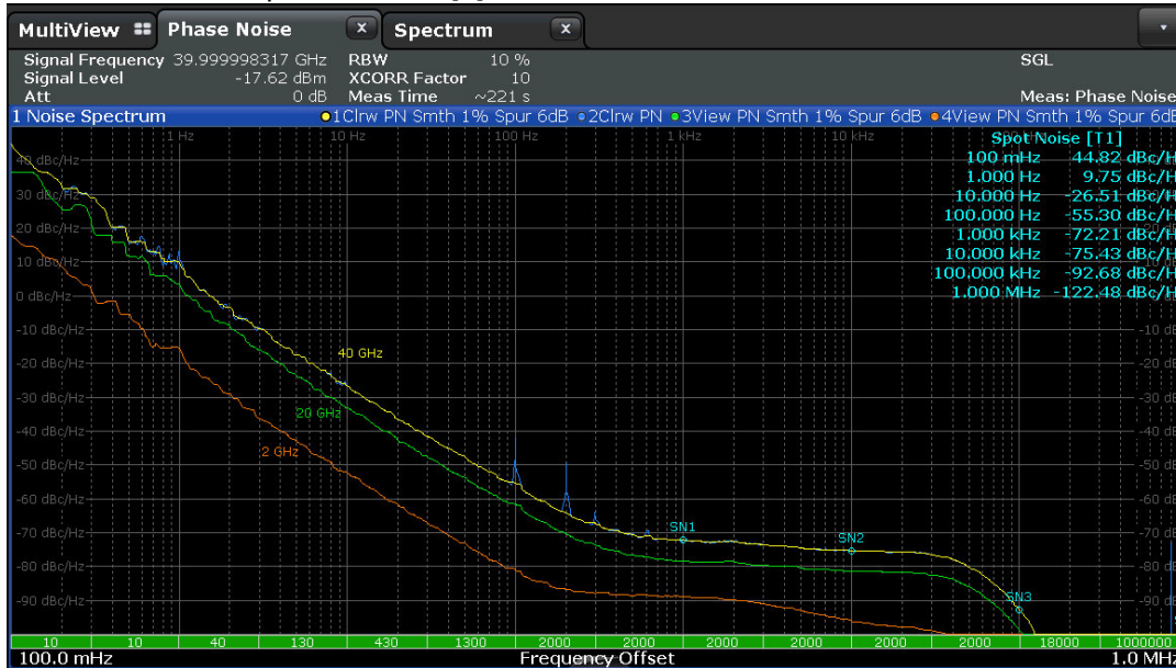
Figure 3: Measurement of a 40GHz source where the spot noise is larger than zero
